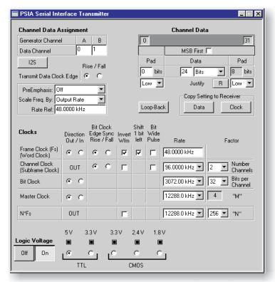
All device parameters are set using soft panels like the one illustrated here. Clock rates, word width and format, data channels and other parameters can be set and saved to allow easy and predictable device tests. Panels are included for transmit and receive functions with the ability to copy settings from one to the other.
