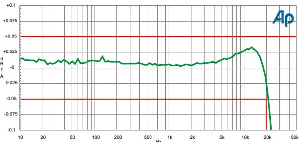
Pass-band response showing flatness out to 20 kHz.
